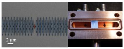
Left: example of a Josephson meta-material we engineer in our lab. It is made of thousands of Josephson junctions and behaves as a "superinductance", which is several orders of magnitude larger than what is usually found in standard electronic circuits. Right: superconducting qubit embedding a superinductance (black rectangle) sitting in its copper microwave cavity. In this specific case, the addition of a superinductance enabled a novel readout mechanism.
